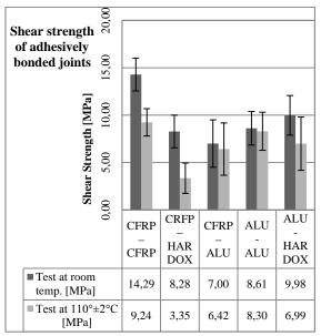
Fig. 6. The shear strength of bonded joints
